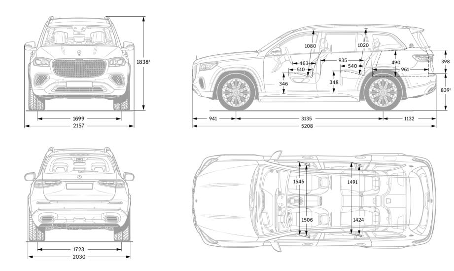
¹With suspension set to "On-Road". All figures in millimetres. The illustrated dimensions are mean values. They are valid for vehicles in basic specification and in unladen condition.
