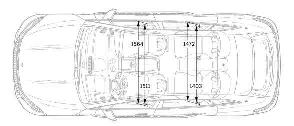
All figures in millimetres. The dimensions shown are mean values. They are valid for vehicles with standard equipment and in unladen condition.
